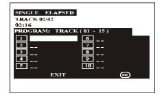
Input the desired tracks using numbers buttons (0~9) on the remote as shown in diagram. If you want to program more than 10 songs, you can highlight ►►I and press ENTER to go to the next page.
